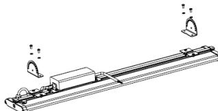
4. Place the luminaire on ceiling brackets with M5x16 screws and washers, adjust pivot angle of turn brackets and tighten M5 screws with torque (6+0.5) Nm.
