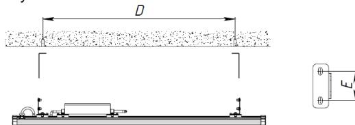
3. Place pivot brackets from hardware kit on a luminaire (2 pcs) with M5x10 screws and washers.
