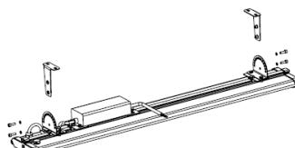
5. Connect mains power to the luminaire with sealed connector (not included) or sealed junction box (not included) according to polarity shown: «L» phase conductor - brown, «N» negative conductor - blue, ground - yellow-green.
